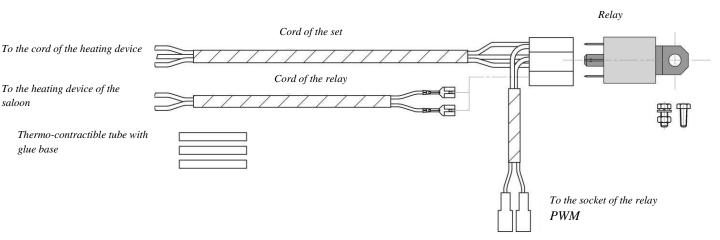
To perform further connection according to the circuit of electrical connections
