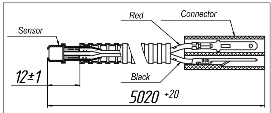
Fig. 23 – Temperature sensor
