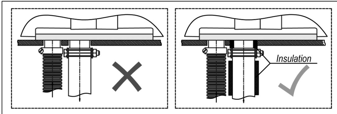
Fig. 12 – Installation of additional heat insulation
