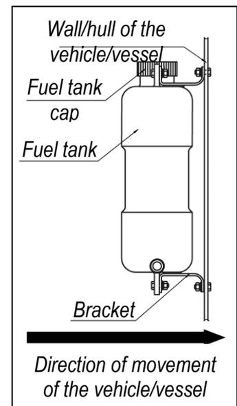
Fig. 16 Installation of the fuel tank
