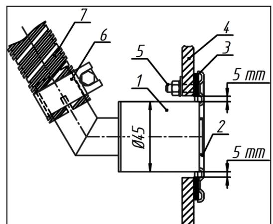
Fig. 13 - Installation of the exhaust pipe
