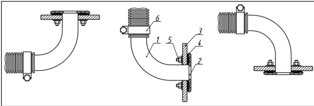
**Fig. 7 - Installation of the air intake pipe**
