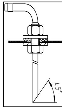
Fig. 15a – Installation of the fuel suction hose
