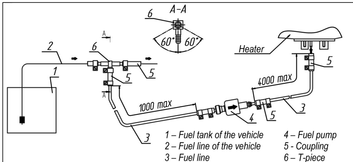
Fig. 17 – Fuel suction using a T-piece
