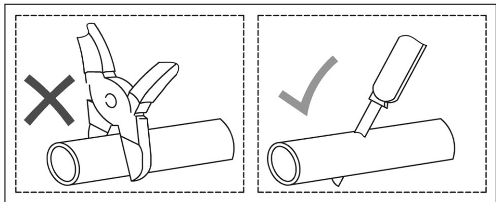
**Fig. 21 - Cutting of the line before installation.**
