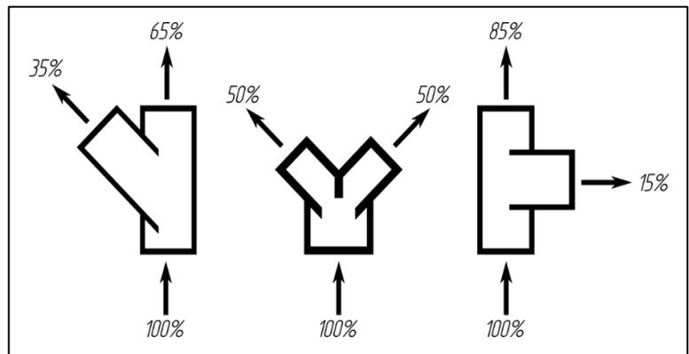
Fig. 25 – Examples of air distribution with different components
