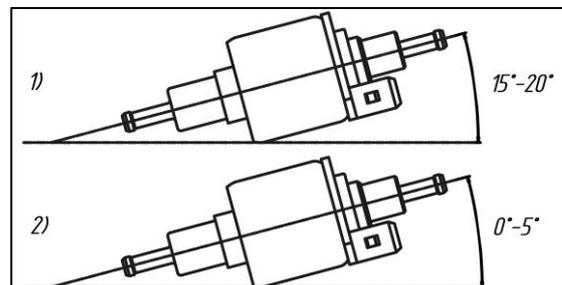
Fig. 18 – Installation angle of TH-9; TH-10; TH-11 fuel pump (1) and Thomas Magnete (2) fuel pump.
