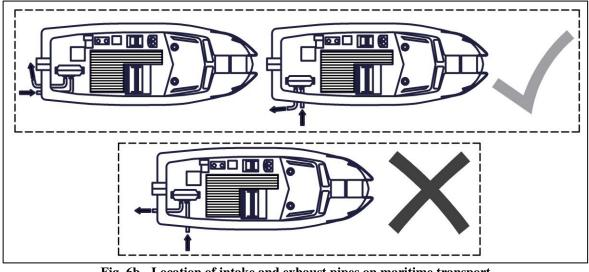
Fig. 6b - Location of intake and exhaust pipes on maritime transport
