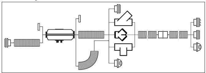
Fig. 26a - Air duct connections for AIR-2D (60mm)
