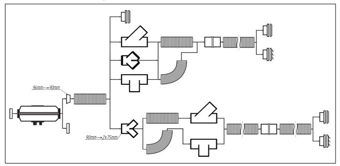
Fig. 26b – Air duct connections for AIR-4D (90mm/75mm)
