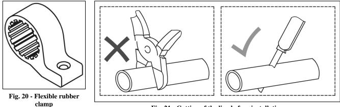
Fig. 21 - Cutting of the line before installation.
