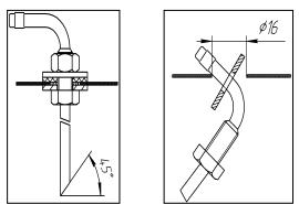
Fig. 15a – InstallationFig. 15b – Installation ofof the fuel suction hosethe washer.
