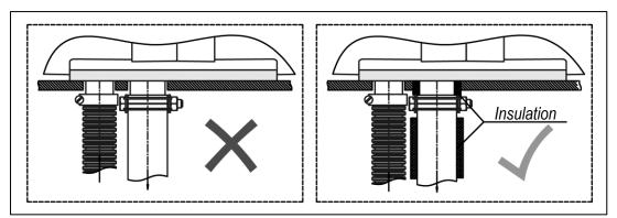
Fig. 12 – Installation of additional heat insulation
