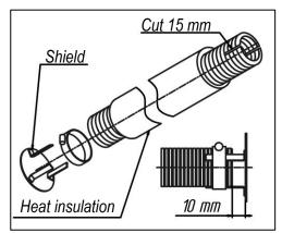
Fig. 9 – Exhaust pipe shield
