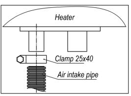
Fig. 4 – Connection of the air pipe to the heater
