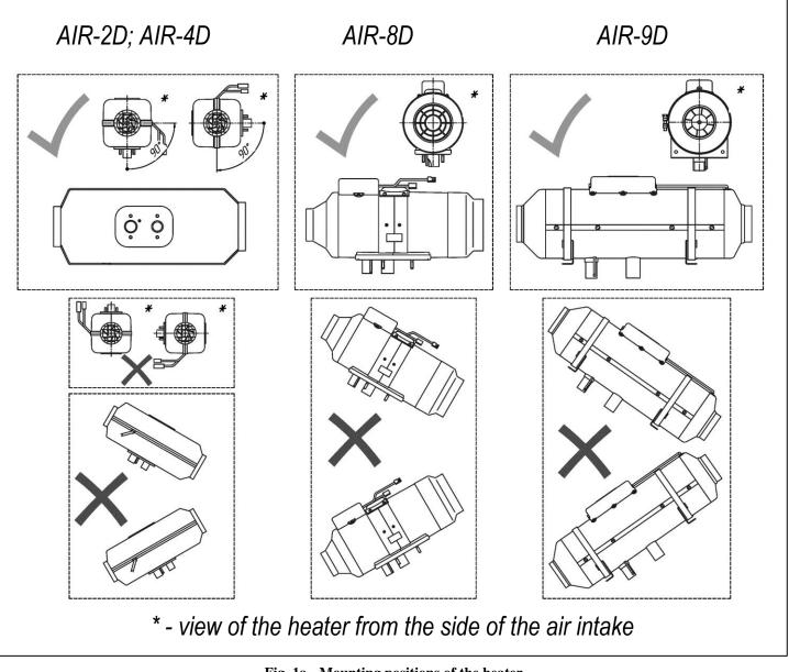
Fig. 1a - Mounting positions of the heater
