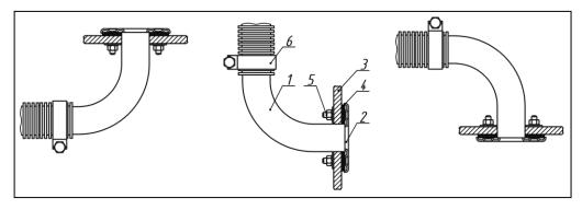
Fig. 7 - Installation of the air intake pipe
