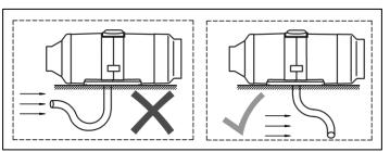
Fig. 5 – Position of air intake/exhaust pipe
