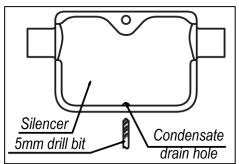
Fig. 10a – Condensate drain hole for horizontal mounting
