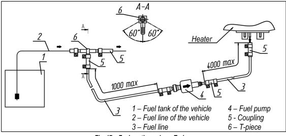
Fig. 17 – Fuel suction using a T-piece
