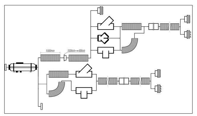
Fig. 26c – Air duct connections for AIR- 9D (100mm/90mm)
