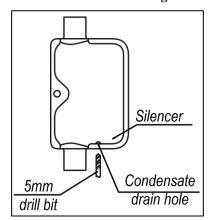
Fig. 10b – Condensate drain hole for vertical mounting
