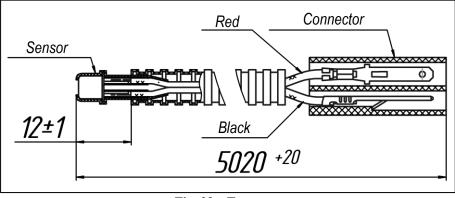
Fig. 23 – Temperature sensor
