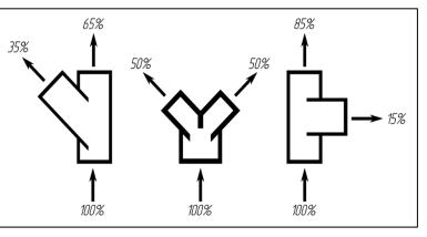
Fig. 25 – Examples of air distribution with different components
