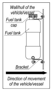
Fig. 16 Installation of the fuel tank
